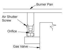
Figure 20 - Air Shutter Adjustment
